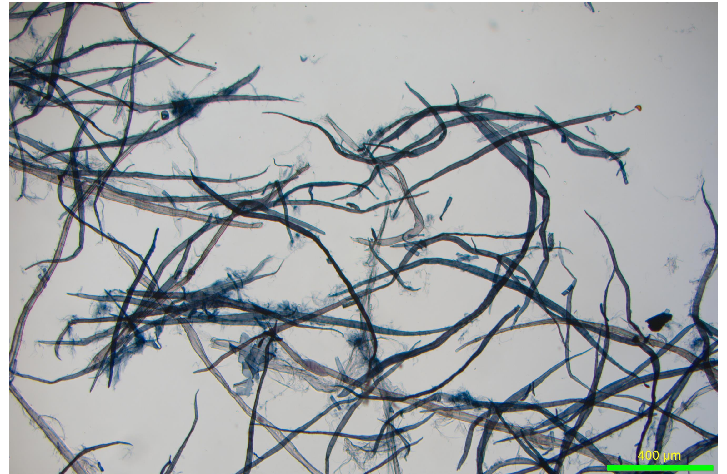
60C SW fillings used for birch refining more crushing (SEL 1.5 J/m, 150 kWh/t)
